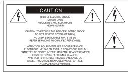
The lightning flash with arrowhead symbol within an equilateral triangle, is intended to alert the user to the presence of unisulated dangerous voltage within the products enclosure, that may be of sufficient magnitude to electric shock to persons. Le symbol clair avec point de fl che intriteur d un triangle quilat ral est utilis pour alerter I utilisateur de la pr sence i int rieur du coffret de vottage dangereux non isol d ampleur suff
