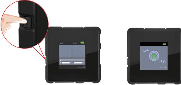
**Step Three:** Turn on the transmitter/s.
